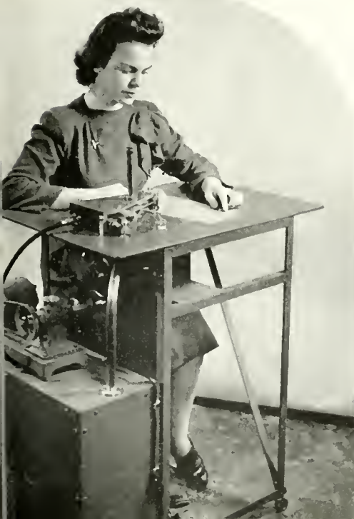
RADIO-FREQUENCY CURRENT TAKES THE PLACE OF NEEDLE AND THREAD IN THE ELECTRONIC SEWING MACHINE (LEFT) AS DEMONSTRATED BY RCA LABORATORIES.
