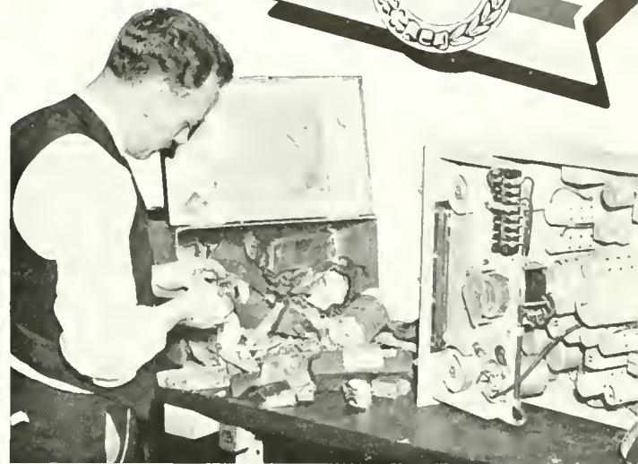
"SUBMERGED" WAS MARKED ON THIS BATTLE-DAMAGED COMMUNICATIONS EQUIPMENT (ABOVE) SENT TO RCA VICTOR FOR RECLAMATION. SEALING TOGETHER PARTS OF MINIATURE TUBES (BELOW) IS ONE OF MANY STEPS IN MANUFACTURING AT RCA VICTOR IN HARRISON, N. J.
